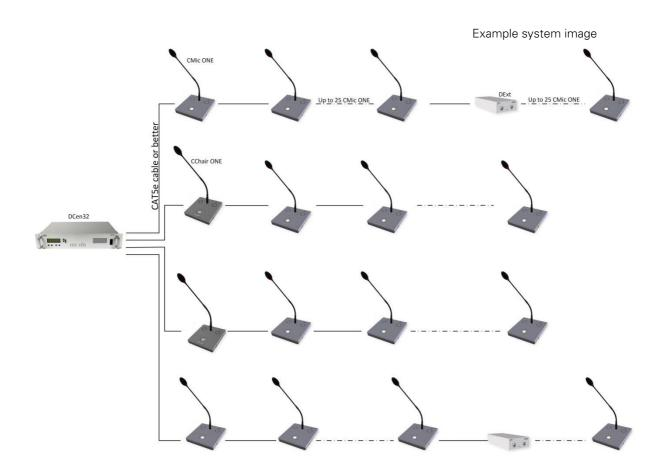
The CMic ONE units are connected to each other by CAT5e cable or better. CMic ONE chains can be extended using the DExt additional power supply.
